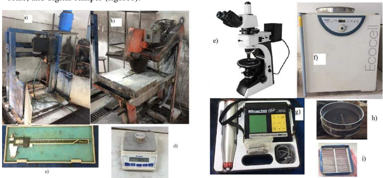
Figure1. Equipments used during the analyses: a) Core drilling machine, b) Cutting machine, c) Digital calliper, d) Scale, e) Polarizing microscope, f) Oven, g) Schmidt hammer, h) Cylindrical sieve, I) Bar sieve
