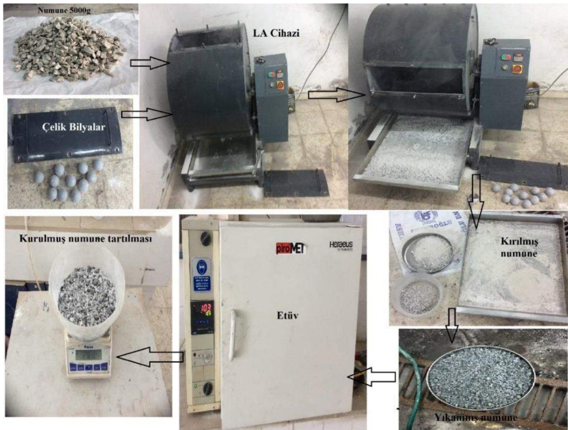
Figure3. Los Angeles test procedure and equipments.
